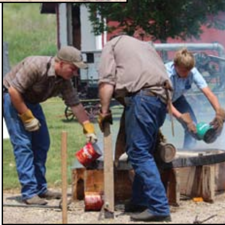
Group 1: Mel Rufs-vold, Kerwin Lund and crew doing the wheelwright demonstration. This is when new wood is put into wood wheels from wagons or equipment. The outside steel band is heated in a ring of fire to expand it to fit over the wood wheel and then is shrunk with cold water to make it fit tight. Look close and see the water boil as they place the wheel in the trough.
