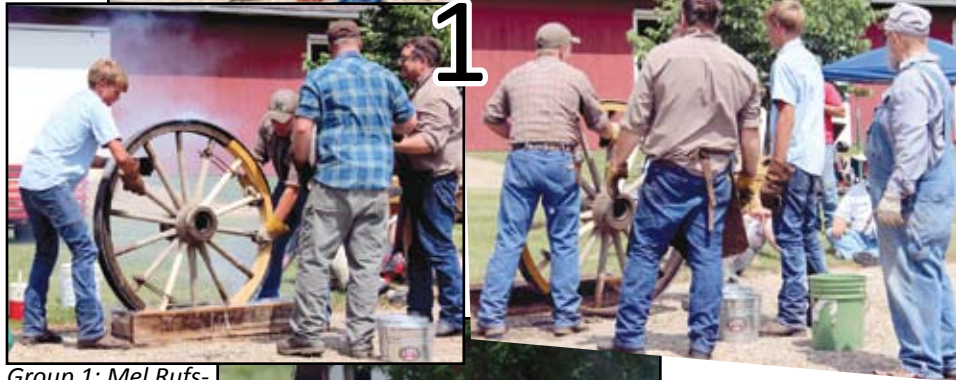
Group 1: Mel Rufs-vold, Kerwin Lund and crew doing the wheelwright demonstration. This is when new wood is put into wood wheels from wagons or equipment. The outside steel band is heated in a ring of fire to expand it to fit over the wood wheel and then is shrunk with cold water to make it fit tight. Look close and see the water boil as they place the wheel in the trough.
