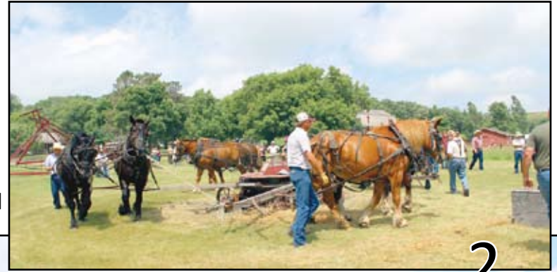
Group 2: Clint Sweet, Lisbon, ND drives the Belgian horses as they walk in a circle powering the unit which provides power to operate the horsepowered threshing machine. Clayton Brennan drives the black team. Four teams drive the unit.
